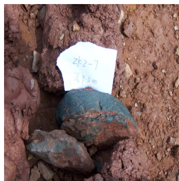
图5 注浆后滑动段土体钻孔抽芯 Fig.5 Drilling drawing-core in sliding zone after grouting
